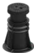
Series 80/31 Surface box "Classic" according to DIN 4056 for distribution valves Height adjustable Cast iron lid Body of PA+
