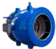
Series 872 Needle valve DN 80-1600 PN 10/16/25/40 Stainless steel DN80-150 Ductile iron from DN200
