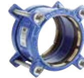
Series 621/10 Supa Plus™ straight coupling Tensile for PE and uPVC pipes DN32-300 PN16 Ductile iron
