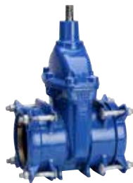
Series 01/70 Supa Plus™ gate valve Tensile for PE and uPVC pipes DN40-300 PN16 Ductile iron
